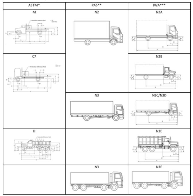
Test Standard Vehicle Image Comparison for 2, 3, and 4 Axle Trucks
